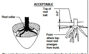
The point where top-most root(s) emerges from the trunk (root collar) should be within the top 2" of substrate. The root collar and the root ball interior should be free of defects including circling, kinked, ascending, and stem girdling roots. Structural roots shall reach the periphery near the top of the root ball.
